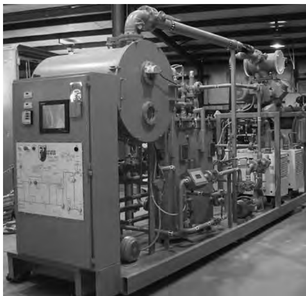
FIGURE 4.5 Vacuum dehydrator oil unit, Model BA-D-H-1800. (Courtesy of Baron USA, Inc., Cookville, TN.)
