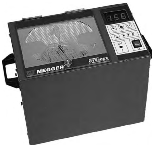
FIGURE 4.2 Oil dielectric test set 60kV. (Courtesy of Megger, Inc., Valley Forge, PA.)
